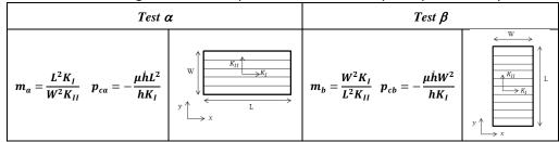
Tab. 1: Positioning of fabrics and parameters for the in-plane permeability tests.
