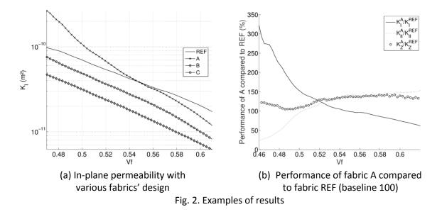
In this study an innovative method has been proposed and used to continuously extract the in-plane permeability coefficients of various fabrics. The results allow to quantify very finely the performance (in gain or loss) of the fabrics with new fabric design parameter over the full range of Vf of interest.
